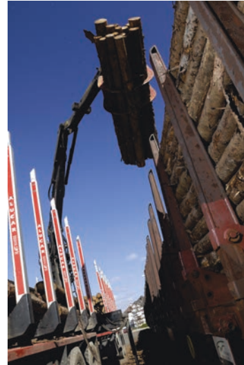
(b) Lorry-mounted crane
