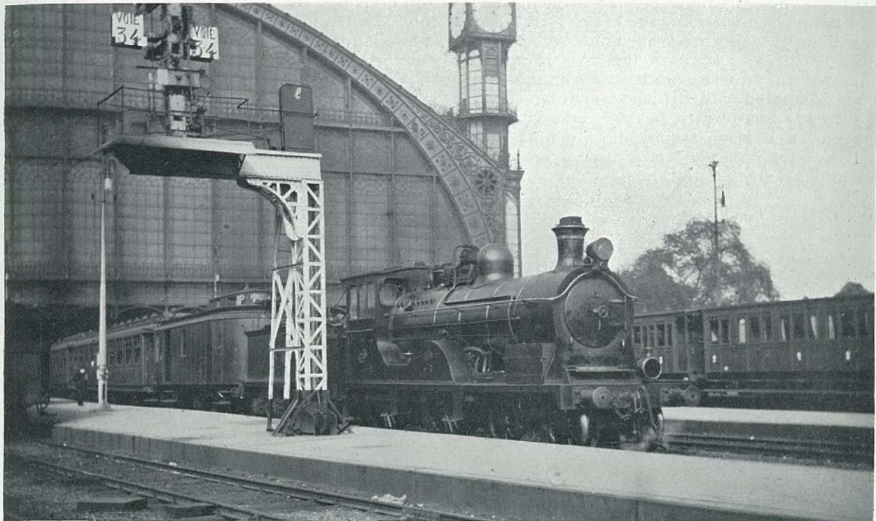
ANTWERP CENTRAL STATION.—Block Train for Brussels, 5 8-Wheeled Bogie Coaches and 2 6-Wheeled Brake Vans, with rounded ends, headed by "Dunalastair" type Locomotive, C. de F. de l'Etat Belge. Photo Loco. Pub. Co. Ltd.
