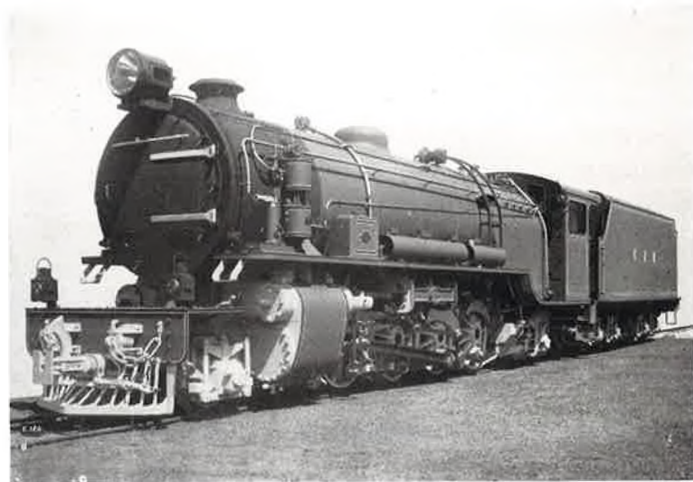
2-8-2 Mikado Locomotive for 80 lb. rail (built by Messrs. Robert Stephenson &amp; Co. Ltd., Darlington)
