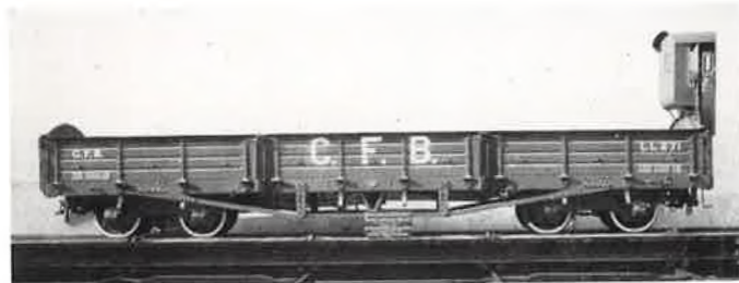
Low sided bogie wagon, Benguella Railway. (Built by the Metropolitan Carriage, Wagon & Finance Coy. Ltd.)
