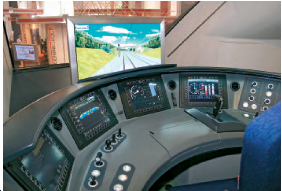
↑ The EUCAB European driver's cab heralds the progressive standardisation of railway rolling stock.
