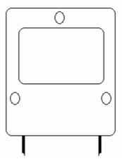
The front lights must optimise train detectability (e.g. to track workers and those using public crossings), provide sufficient visibility for the train driver (illumination of the line ahead, lineside information markers/boards, etc) by night and during low light conditions and shall not dazzle the drivers of oncoming trains.
