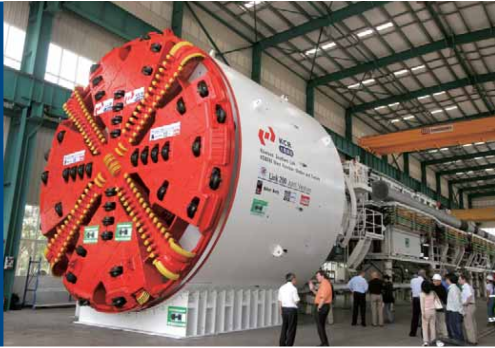
This tunnel boring machine was designed specifically for the Kowloon Southern Link
