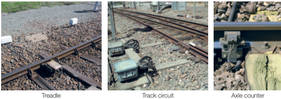
Figure 1.5: Examples of outdoor equipment for track vacancy proving
