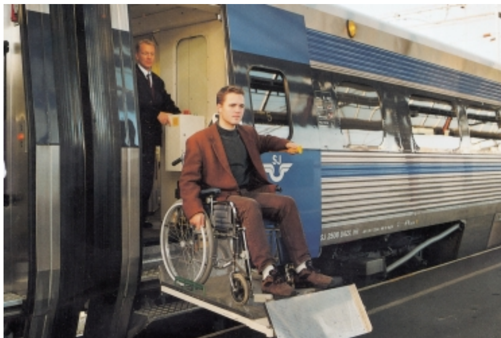
Figure 4.4. Platform lift – SNCF railways – FR
