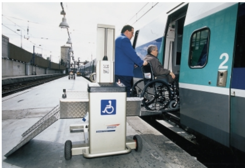
Figure 4.4. Platform lift – SNCF railways – FR
