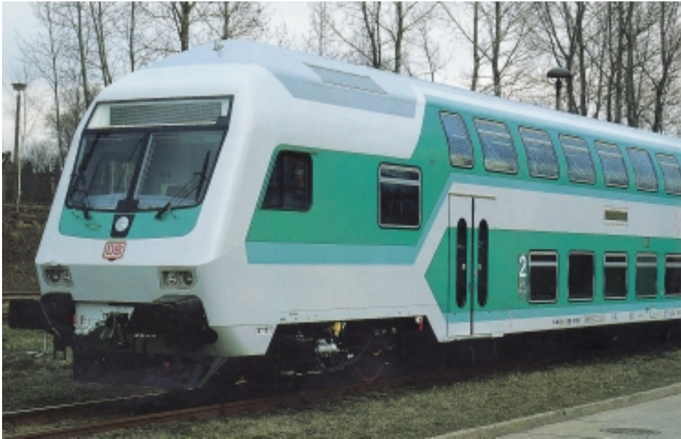
Double-deck driving trailer, type DBbzf 761 (Bremen)
