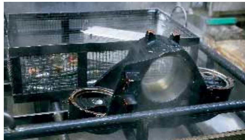
Washing machine Steel components of a diesel multiple unit going through the wash in Kassel.
