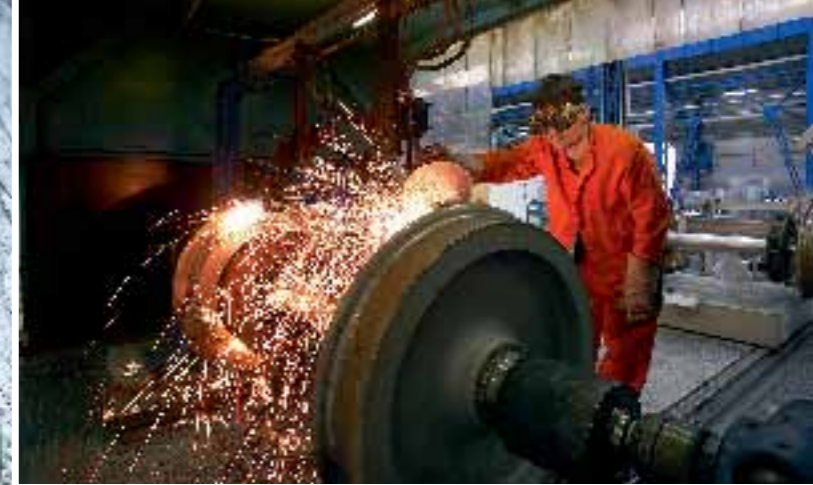
Iron core Before a wheelset is reconditioned in DB's Kassel depot, a technician takes it apart using a cutting torch.
