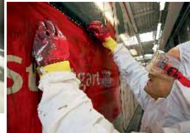
Next please Maintenance of S-Bahn trainsets is performed in Plochingen. Graffiti is removed using special detergents.
