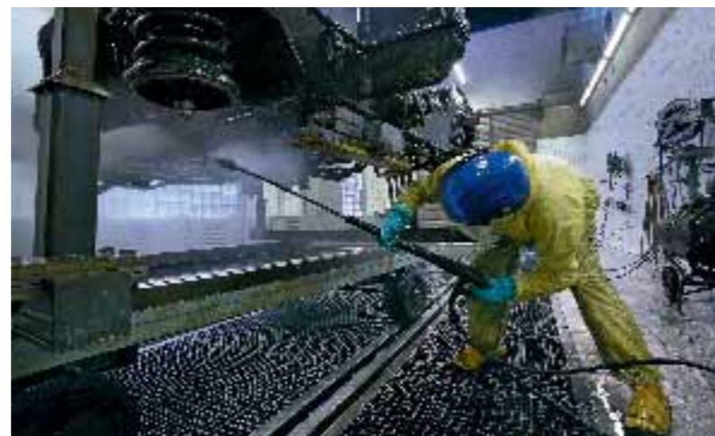
Washing machine Steel components of a diesel multiple unit going through the wash in Kassel.
