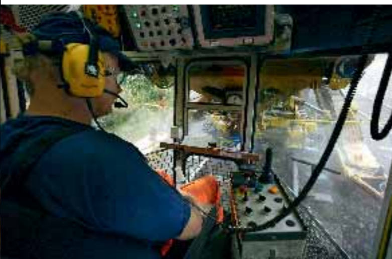
Track bed Bit by bit, a new track appears. View into the cab of the tie laying unit on the track renewal train (below).
