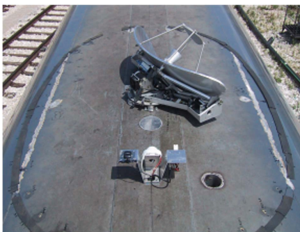
Figure 12 : Roof antenna and radom mounted on a Thalys train
