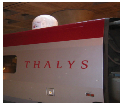
Figure 12 : Roof antenna and radom mounted on a Thalys train
