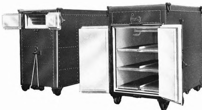
Fish traffic container with ice compart- ments for refrigeration. These containers have been supplied to the National Rail- ways of Colombia.
