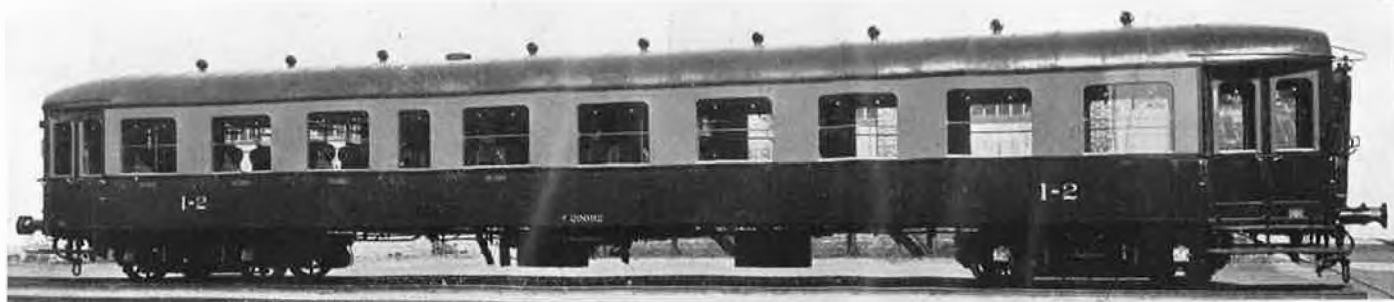
Above: First and second class composite coach for internal express trains. Note large double vestibule end doors
