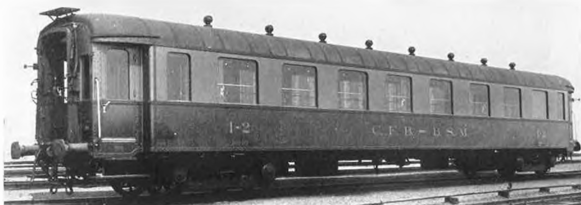
First and second class all-steel composite coach of the side-corridor type as used for international services
