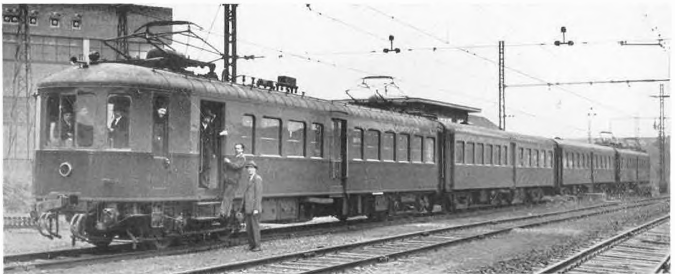
Four-car 3,000-volt d.c. electric train as used on the newly electrified railway between Brussels and Antwerp on the Belgian National Railways system
