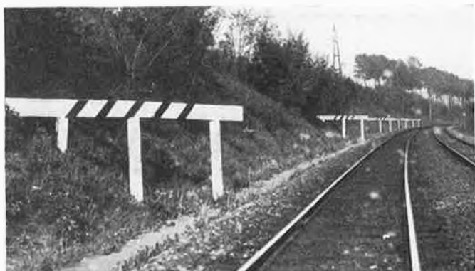
Fig. 1—Approach warning boards in front of a distant signal
